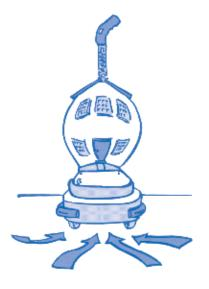
R adon is a naturally occurring radioactive gas produced by the breakdown of uranium in soil, rock, and water. Air pressure inside your home is usually lower than pressure in the soil around your home's foundation. Because of this difference in pressure, your home acts like a vacuum, drawing radon in through foundation cracks and other openings.
